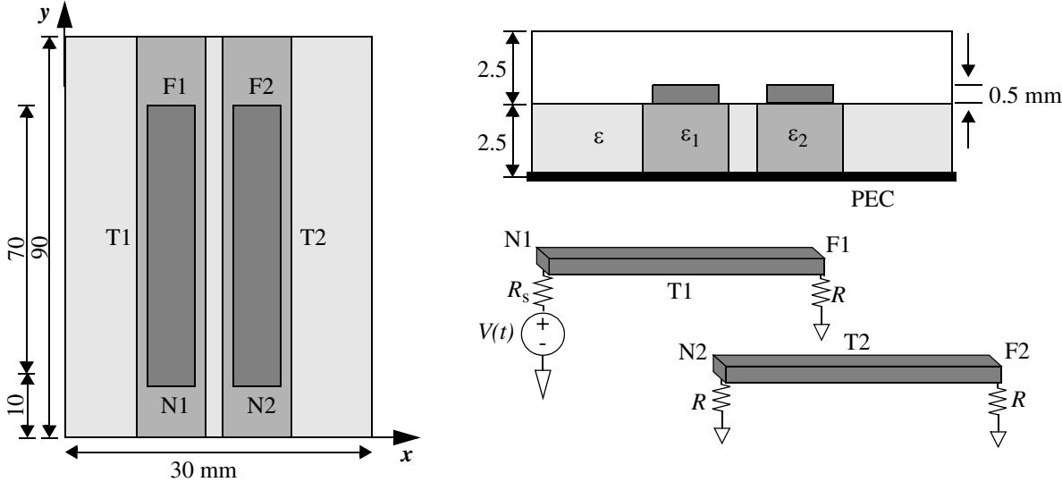
The substrate is made of alumina (*i.e.* a ceramic  $\epsilon = 10$ ) and the dielectric strips have the following dielectric constant values:
